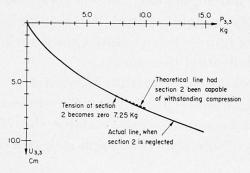
Fig. 17. Curve of  $U_{3,3,3}$  versus  $P_{3,3}$ .
