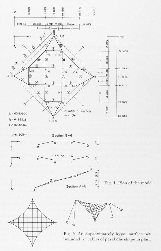
of inner joints. In this case J=12, but there are only 28 bars instead of the 36 necessary for a determinate system. In the case of prestressed cables, however, a certain degree of stabilization is provided, as shown for similar suspended roofs [3]. The higher the prestress, the stabler the system.
