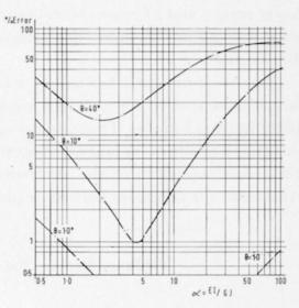
Fig. 3. Simulation of curved member by an equivalent straight uniform member. Percentage error in torsion stiffness.
