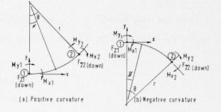
member are given below, where the upper sign refers to positive, lower to negative curvature of the curved member as defined in Fig. 13.
