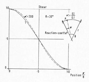
Fig. 9. Influence lines for end reaction in a curved girder with  $\theta = 30$  degrees.
