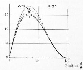
Fig. 8. Influence line for bending moment in a curved girder with  $\theta = 30$  degrees.
