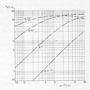
Fig. 4. Simulation of curved member by an equivalent straight uniform member. Percentage error in shear stiffness.
