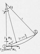
Fig. 15. Simulation of curved member by an equivalent straight member.
