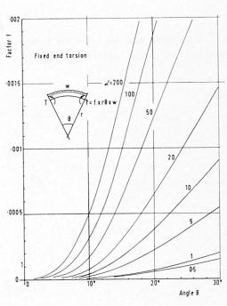
Fig. 6. Values of fixed end torsions in a curved girder under uniformly distributed load.
