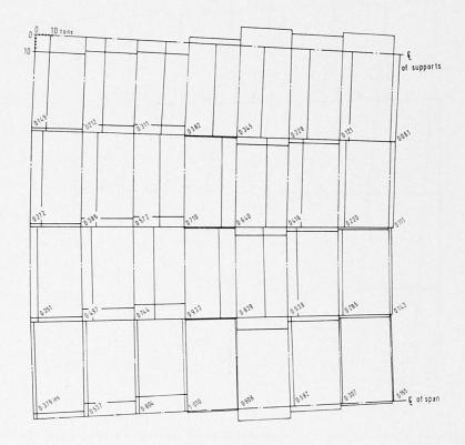
Fig. 12. Lofthouse Interchange — Distribution of shears and deflections.
