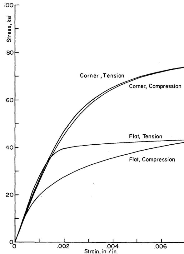
Fig. 3. Stress vs strain, flats and corners, longitudinal, type 304 stainless steel, annealed and skin passed.
