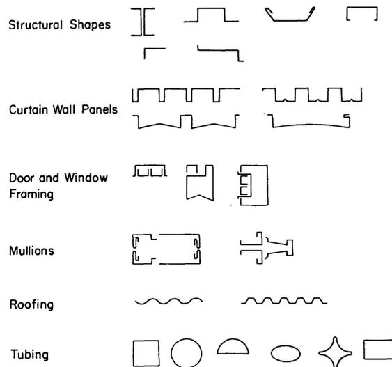
Fig. 1. Typical stainless steel sections.
