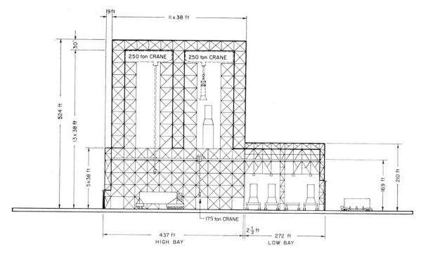
Fig. 16. North-South Section along transfer aisle of V.A.B.
