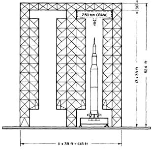
Fig. 14. North-South Section through Assembly Chambers of V.A.B.
