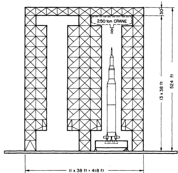
Fig. 14. North-South Section through Assembly Chambers of V.A.B.
