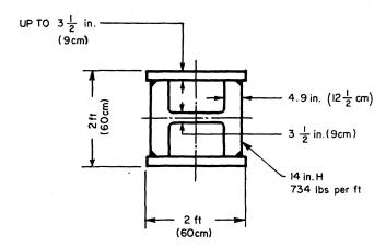
Fig. 21. Section of welded column.
