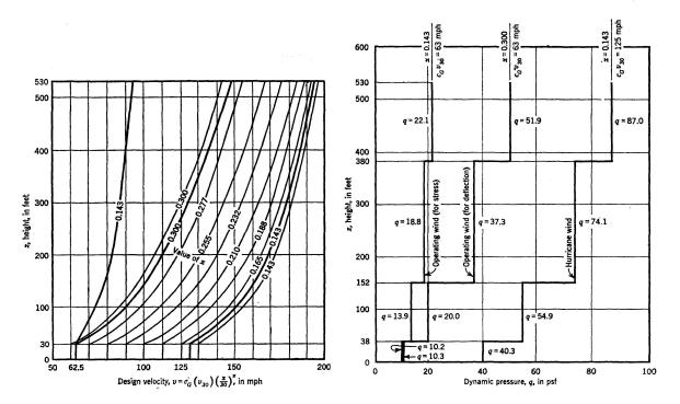
Fig. 18. Wind velocity as a function of height.
