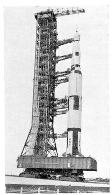
Fig. 3. Mobile launcher with space-vehicle.
