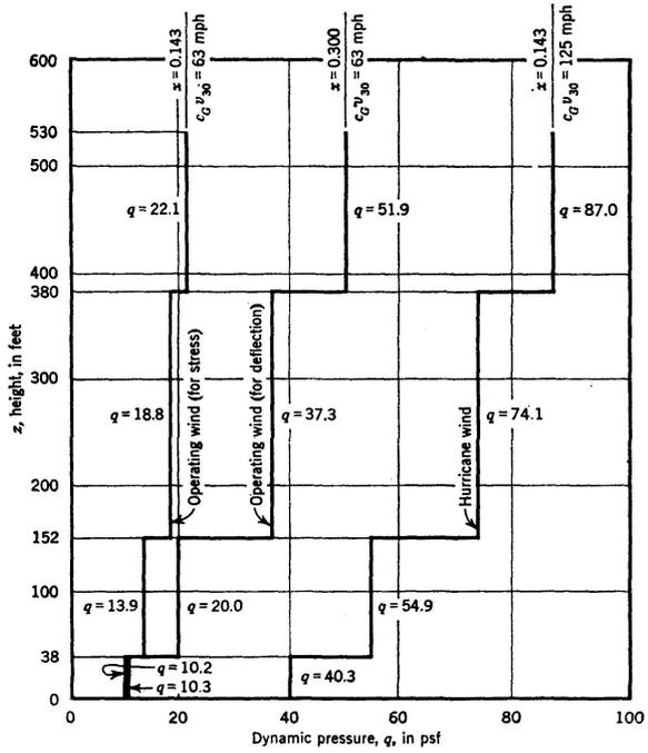
Fig. 19. Wind pressure as a function of height.
