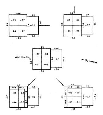
Fig. 20. External pressure coefficients.
