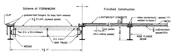
Fig. 27. Section through typical slab of V.A.B., showing form work.
