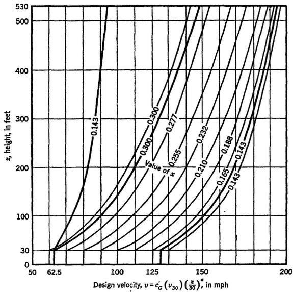
Fig. 18. Wind velocity as a function of height.
