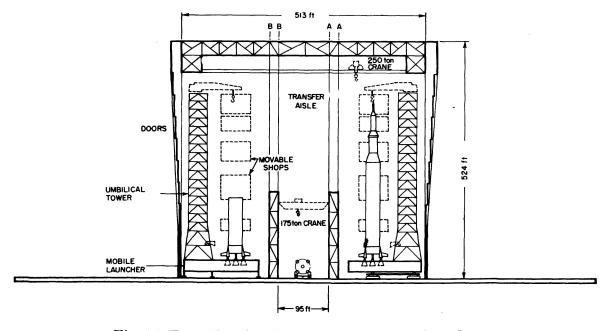
Fig. 15. East-West Section through Assembly Chambers.
