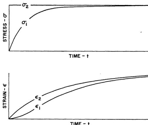
Fig. 2. Creep strain corresponding to two stress histories.
