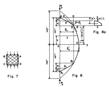
Calling the size of the hinge block (Fig. 2a) k'l and the yielded length of the member from the end to the middle of the plane DE, point N, kl the angle between the original direction of the axis and the line ON is found as
