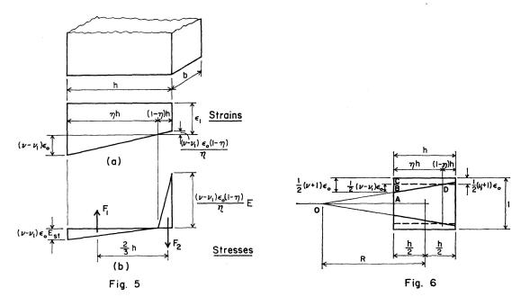
Fig. 6 shows the deformation to a curvature c=1/R of a unit length of the column. From similarity of the triangles OAB and BCD
