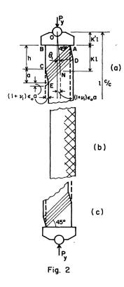
Deviations from the general pattern were frequent. Thus significant deflection was often observed in the direction inconsistent with the hinges, with formation of triangular wedges on the faces parallel to the hinge. One  $1'' \times 1'' \times 10''$  column even failed completely while undergoing such unexpected deformation.
