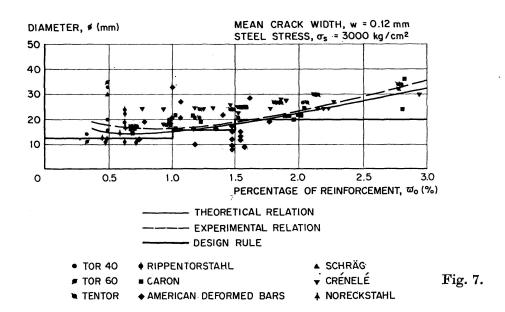
The dotted lines representing the mean of the experimental values obtained agree well with the theoretical lines. As the scatter of the individual results is considerable, it is advisable for practical purposes to limit the diameters to values below the thick line also indicated in fig. 6 and 7. It should be noted that the experimental results which do not satisfy this limit correspond to tests in which the cover considerably exceeds the usual values.
