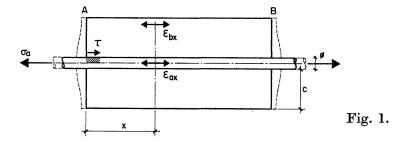
It is also easy to justify the proportionality of the mean distance between cracks to the ratio between the diameter of the bars and the percentage of reinforcement which is equivalent to the ratio of the area of concrete under tensile stress  $B_t$  to the perimeter of the bars p.
