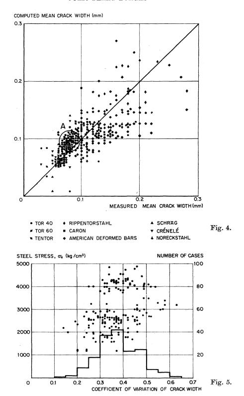
The mean value of 1.03 was obtained for all the results considered and no significant change of the mean values was noticed for increasing values of the steel stress. The coefficient of variation decreases from 0.32 to 0.23 as stresses increase from 2100 to 4000 kg/cm<sup>2</sup>.
