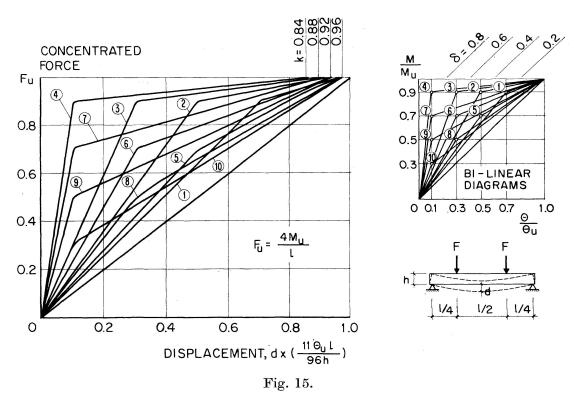
for bi-linear diagrams with the same area, force-displacement diagrams end at almost the same point.
