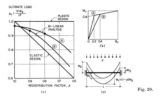
the usual percentages  $(\tilde{\omega}_0 < 3\%)$  and of steel 40 in percentages  $\tilde{\omega}_0 < 1\%$ . Diagram B is on the safe side for percentages  $\tilde{\omega}_0 < 2.5\%$  of steel 40 and can be considered to correspond to the usual percentages of steel of higher quality.
