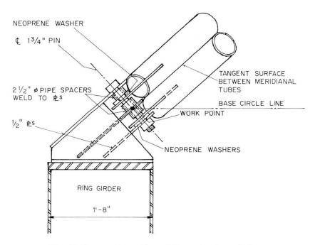
Fig. 9. Connection of meridians to ring girder.
