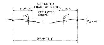
Fig. 8. Developed deflection curve of part of ring girder.
