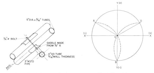
Fig. 3. Typical node showing offset hoop.
