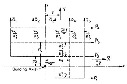
Fig. 4a. Frame arrangement and applied loads.
