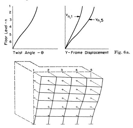
Fig. 6b. Displacements of front face of building.
