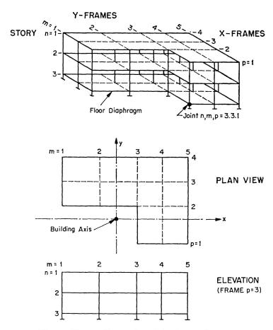
Fig. 1. Three dimensional building frame.
