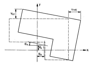
Fig. 4b. Story and frame displacements.
