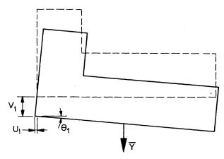
Fig. 5b. Displacement of top story.
