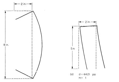
Fig. 4. Deformed cross section of buckled channel — example 3.
