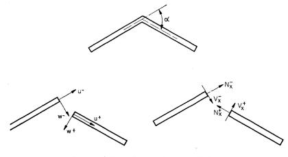
Fig. 3. Transformations at Joint.
