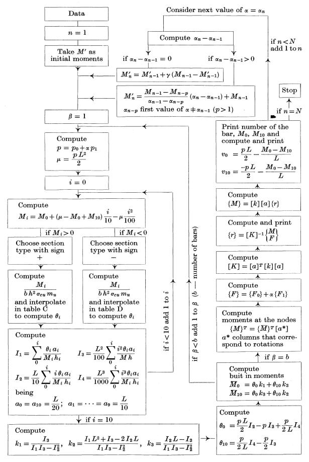
Fig. 11. Flow-chart for non-linear structural analysis.
