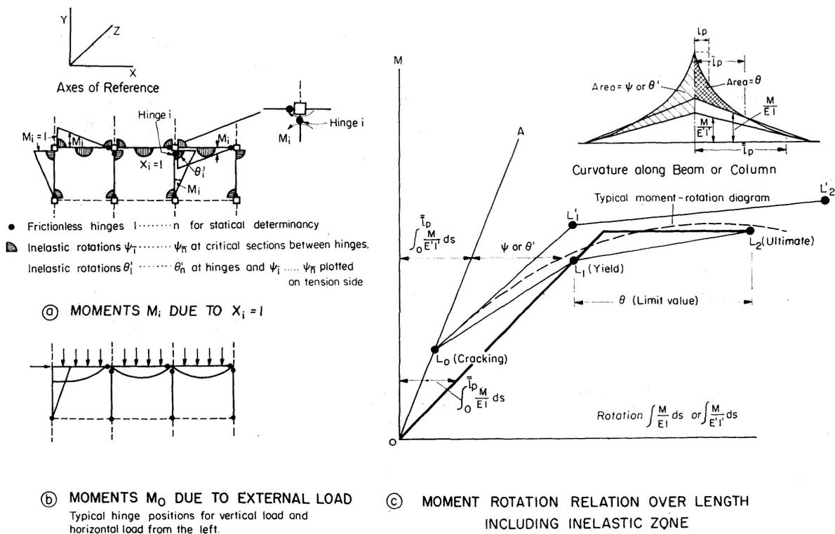
Fig. 1. Typical Basic Characteristics of a Frame.
