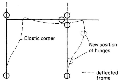
Fig. 4. Deformation of Unstable Frame.
