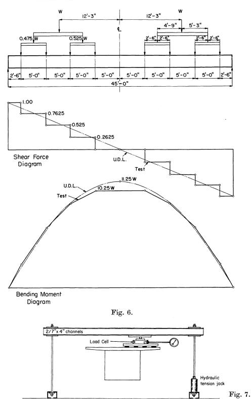
A general arrangement of the concentrated loading (H.B. type to B.S. 153) is shown in Fig. 7 the wheel contact areas being simulated by  $^1/_2$  in. thick rubber pads cut to scale size and loaded through a 1 in. thick steel plate. For the "H.B." loadings the load was measured directly by a resistance gauge load cell.
