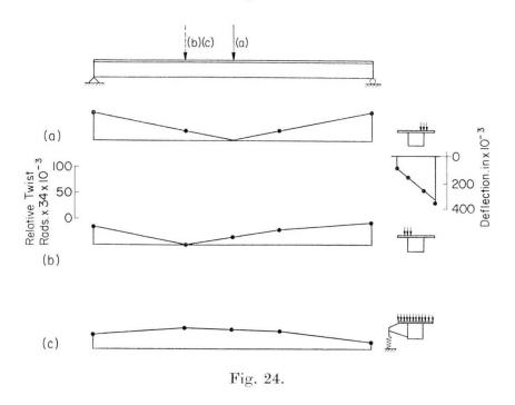
The differential deflection between the edges of the box section is a measure of the torsional twist and Fig. 24 shows the values from which the effective torsional stiffness is calculated as follows
