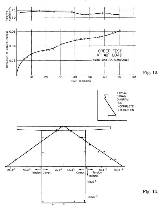
showing a modular ratio of 8. However, this value of the modular ratio gives a neutral axis depth of 6.5 in. whereas the measured depth is 9 in. below the top of the steel. Hence it is apparent that full interaction is not realised although the relative movement of slab and box was not measurable with the  $^{1}/_{1000}$  in. slip gauges.
