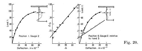
are so small compared to the initial values that Southwell's [2] method for estimating the buckling load was not reliable. However the results selected and shown in Fig. 20 do indicate a critical load to be of the order of 140 t. It is to be noted that the curves plotted for point 2, in Fig. 20 include the overall deflection of the stiffener assembly. This compares with the theoretical value for a simply supported panel buckling in shear of 167 t.
