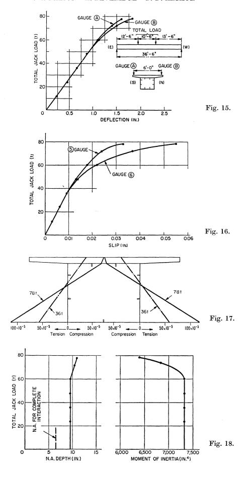
nearer support. At failure the strain gauges on the bottom flange showed no definite departure from linearity and indicated a stress of 18 t/in.<sup>2</sup>. The total force transmitted through the stude at failure was 110 t giving a shear stress on the 220 stude of 18.2 t/in.<sup>2</sup> The shear strength of the stude when tested independently was 20 t/in.<sup>2</sup>.
