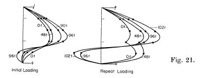
After the weld failure at 102 t there was a large permanent buckle at gauge 4 which was hammered in after the girder had been repaired. The plate profile under the repeat loading shows the return of this bulge after 72 t. At 90 t the buckles in this panel were obvious to the eye and final collapse occurred at a load of 117 t.
