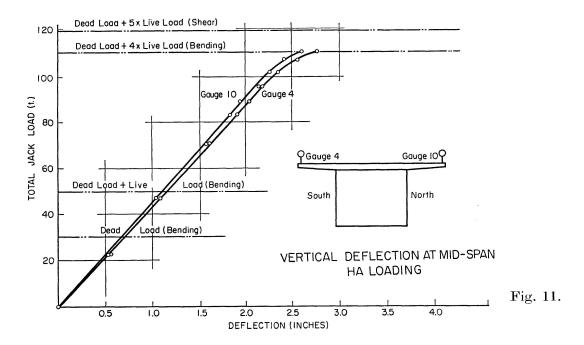
Calculation of the probable deflection due to the shear stresses in the web shows that shear accounts for about 8% of the total deflection and this has been allowed for in the above calculation of I.
