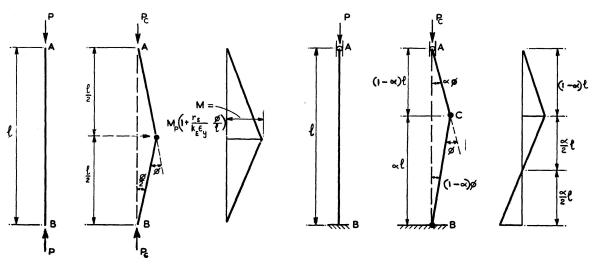
Fig. 6. Solution for pin-ended strut.
