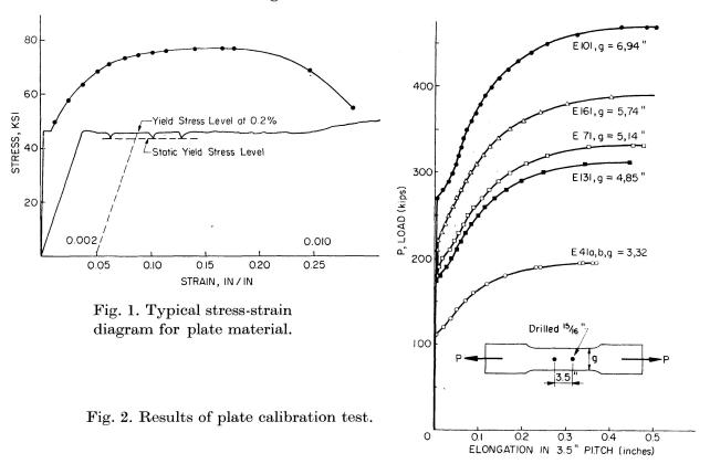
The plate material was purposely ordered near the minimum requirements specified by ASTM for A 440 steel.
