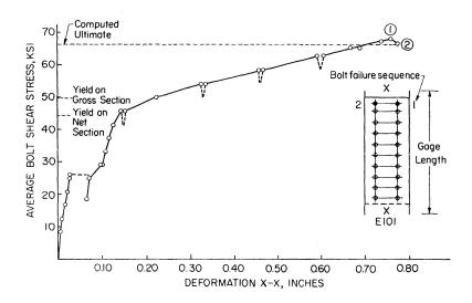
Fig. 5. Typical load-deformation curve.
