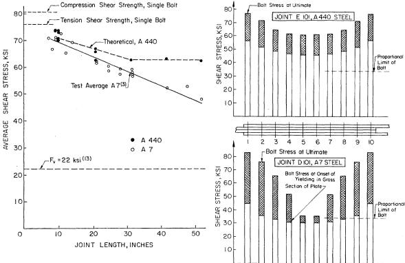
Fig. 9. Comparison of A 440 steel butt joints and A 7 steel butt joints.
