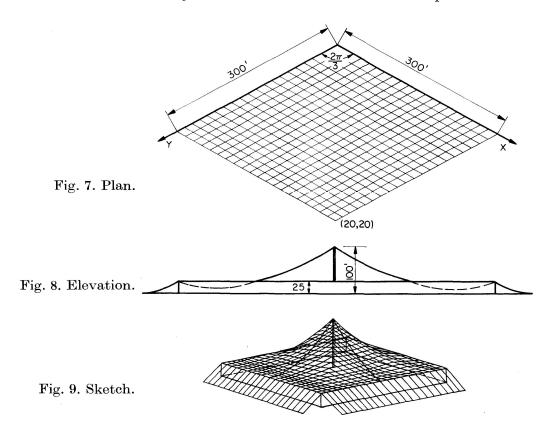
load at the center. The results were combined so as to match the given displacement due to a pole at the center,  $W_t(10, 10) = -75.0$ . (Both fields contain the cable tension as a linear factor; therefore, it is not necessary to duplicate their evaluation in order to study effect changes in that parameter.) The double series, (16,17) and (19) where used primarily, with "spot" checks performed by use of the single series, (25) and (26). The results were identical.
