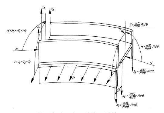
Fig. 6. Loads Acting on Differential Element.
