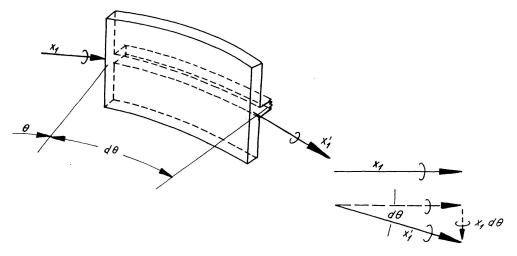
Fig. 4. Vector Analysis of Twisting Displacements of Inner Flange.
