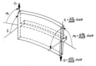
Fig. 5. Internal Tractions Acting on Inner Flange.
