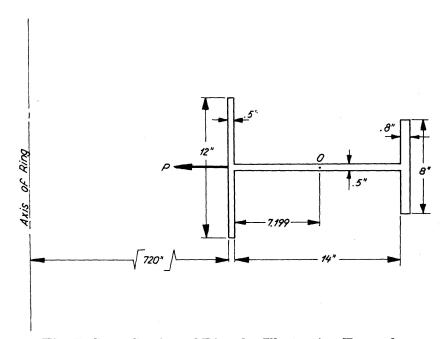
Fig. 7. Cross Section of Ring for Illustrative Example.
