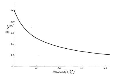
Fig. 11. The mechanism line for a rigid-plastic, simply supported circular plate in compression.
