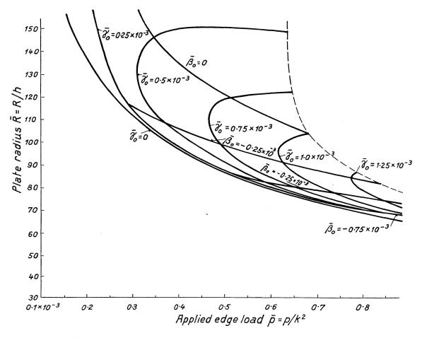
Fig. 6. Plate size vs. Edge load for the clamped elastic plate.
