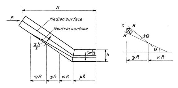
Fig. 9. A general mechanism for the simply supported circular plate in compression.
