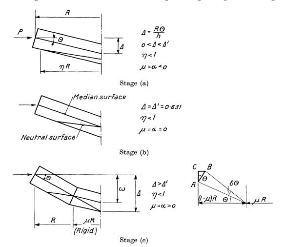
Fig. 10. Unloading of a rigid-plastic, simply supported circular plate.
