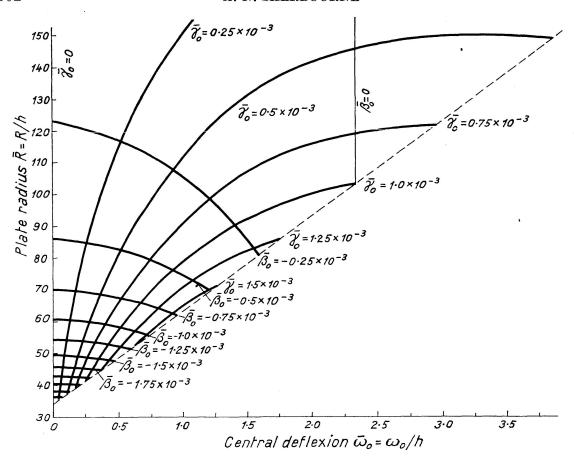
Fig. 8. Plate size vs. Central deflexion for the clamped elastic plate.
