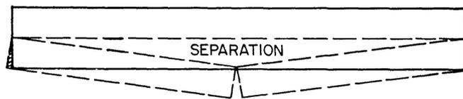
Fig. 6b. Kinematic Picture of Collapse for Load Applied at Mid-Height.
