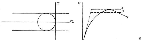
Fig. 3. Mohr's Circle Envelope with Tension Cut-Off.
