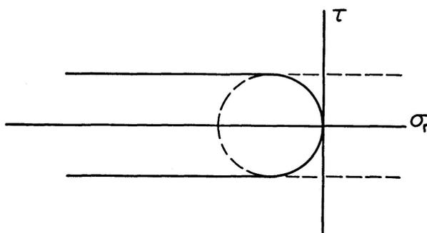
Fig. 3. Mohr's Circle Envelope with Tension Cut-Off.
