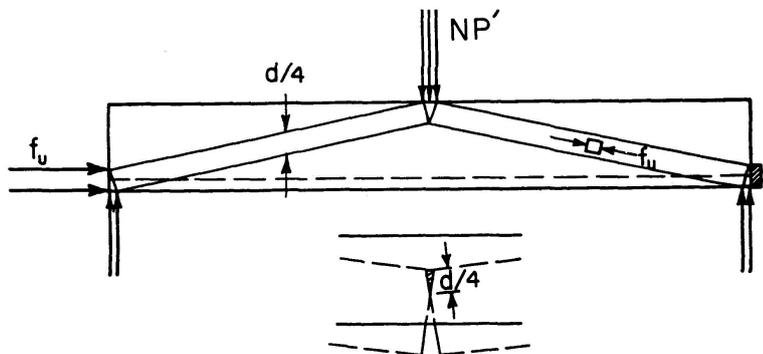
Fig. 8. Less Steel and Less Dependence on Concrete.
