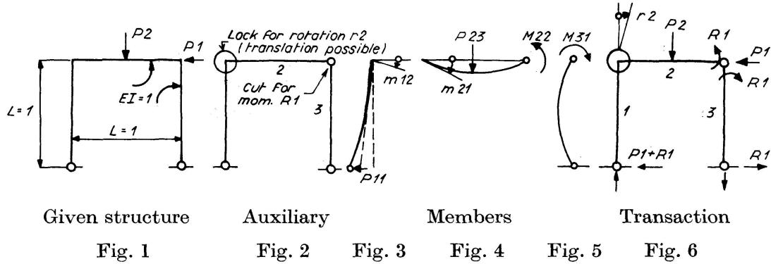
The frame in Fig. 1 is given. It is locked and cut as in Fig. 2 to form an auxiliary, using the members Fig. 3, 4, 5. This is determinate because it is possible by statics and kinematics only to find as in (11) the transaction  $A$ :
