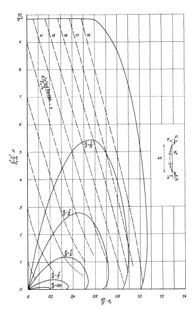
Fig. 5. Relation between the compressive load P and the angle of rotation  $\varphi_v$  of an end of a compression member made of a material having no tensile strength, which is submitted to loads of equal eccentricity at both ends. The full-line curves represent the relations which are obtained when the eccentricity e has certain constant values, while the dash-line curves refer to the relations which are obtained when the edge stress has certain constant values.
