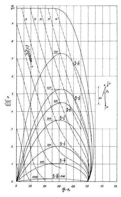
Fig. 2. Relation between the compressive load P and the angle of rotation  $\varphi_v$  of an end of a compression member made of a material having no tensile strength, which is submitted to an eccentric load at one end and to a central load at the other end. The full-line curves represent the relations which are obtained when the eccentricity e has certain constant values, while the dash-line curves refer to the relations which are obtained when the edge stress has certain constant values.
