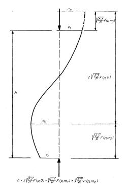
Fig. 7. Elastic Curve of a Compression Member Made of a Material Having no Tensile Strength.
