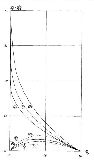
Fig. 3. Relation between the transverse load H and the compressive load P for compression members under the conditions of loading shown in Figs. 1 and 2. The abscissa represents  $\frac{Hh}{Pd}$  for the full-line curves and  $\frac{Hh}{PEd}$  for the other curves. The curves are marked in accordance with the table below.
