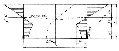
Fig. 14. Free-Body Diagram of the Beam portion Between Two Adjacent Wrinkles.
