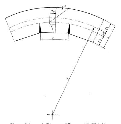
Fig. 8. Schematic Picture of Beam with Wrinkles.
