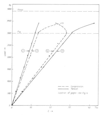
Fig. 5. Strains at Mid-Section of Beam No. 1 AD 1.
