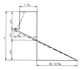
Fig. 10. Assumed Stress Distribution at Ultimate Load.
