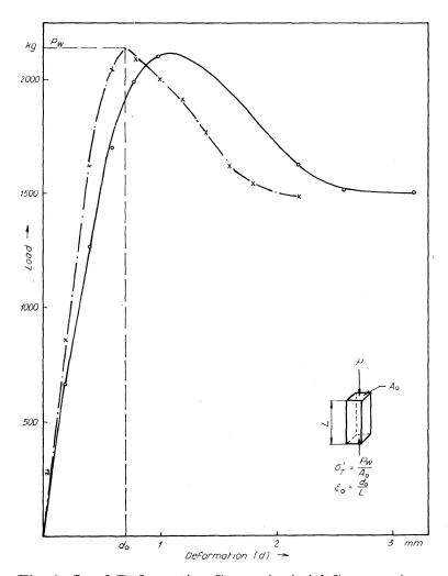
Fig. 9. Load-Deformation-Curves in Axial Compression.
