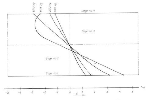
Fig. 4. Strains at Mid-Section of Beam No. 1 AD 1.
