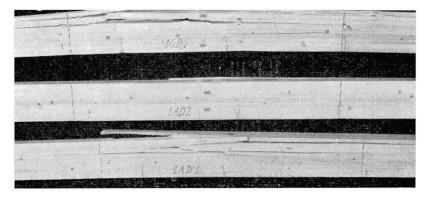
Fig. 6. Beams Loaded to Failure.
