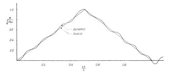
Fig. 4. Bending Moment at x/L=0.5 (plotted against time). L=1127.5 in., v=960 in./sec, P/W=0.5, K/W=3.6545472/in.
