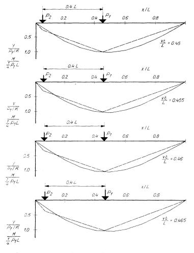
Fig. 3. Successive Instantaneous Bending Moment Diagrams --- and Deflection Curves --- (obtained from the difference equations)  $L=360 \text{ in., } v=803.019 \text{ in./sec}, \ K/W=3.6545472/\text{in., } P_1/W=P_2/W=0.5.$
