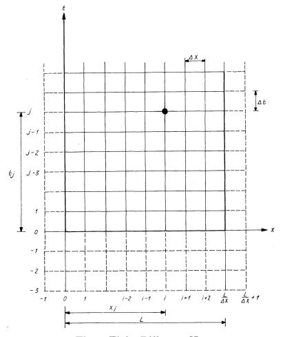
Fig. 1. Finite Difference Net.
