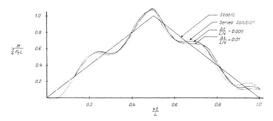
Fig. 2. Bending Moment at x/L=0.5 (plotted against time). L=360 in., v=803.019 in./sec, K/W=3.6545472/in., P/W=0.5.
