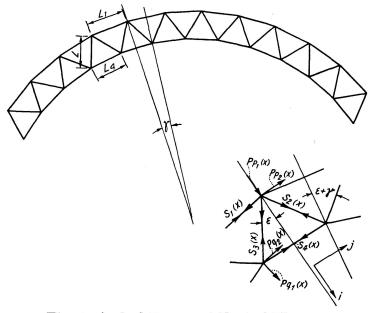
Fig. 4. Arched Truss and Typical Element.
