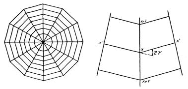
Fig. 1b. Polar Lattice and Typical Element.
