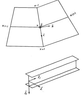
Fig. 3. Typical Element and Member Reference Frame for Conical Lattice.
