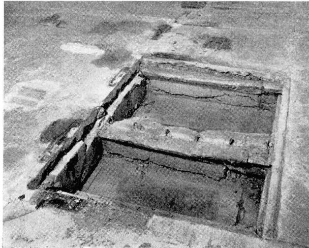
Fig. 7. Box-Section Bridge — Loading No. 7 — Shear Failure in Webs of Beams and Diaphragms.
