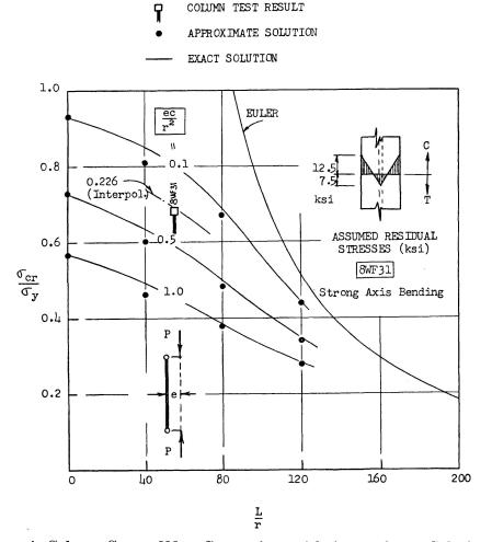
Fig. 9. Eccentric Column Curves [3] — Comparison with Approximate Solution and Tests.
