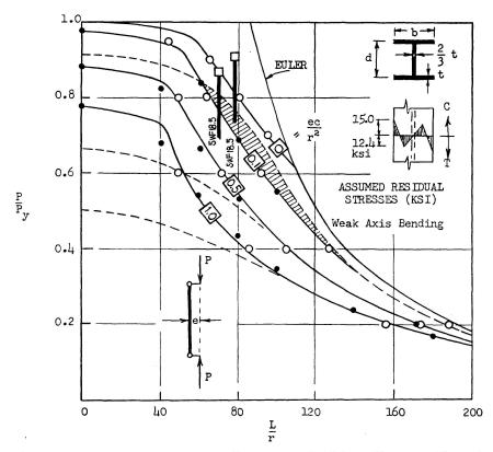
Fig. 6. Axial and Eccentric Column Curves — Cold Bending Residual Stresses.
