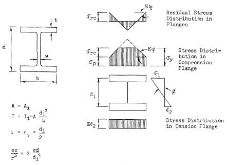
Fig. 7. Actual and Idealized Section with Stress Distribution.
