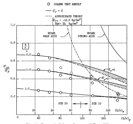
Fig. 10. Eccentric Column Curves and Tests [5].
