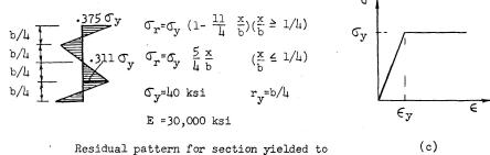
hesidual pattern for section yielded to 1/4 depth prior to unloading
