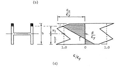
Fig. 2. Residual Stress and Applied Stress in Steel Column.
