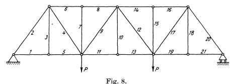
**Example 2: Statically Indeterminate Truss**
