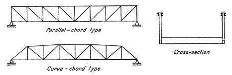
Fig. 1. Typical Pony-Truss Bridges.
