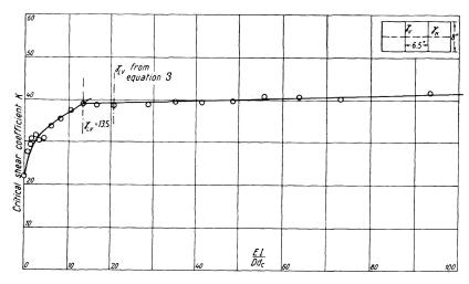
Fig. 4. Results Obtained with Vertical Stiffeners at 6.5" Centres on Webplate Having a Clear Depth  $d_c$  of  $8" \cdot \gamma_H = 9.55$ . Varying Size of Vertical Stiffeners.
