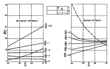
Fig. 8. --- Empirical Relationships. Equation 3 for Vertical Stiffeners. Equation 5 for Horizontal Stiffeners. —— Design Law in DN 4114<sup>12</sup>.
