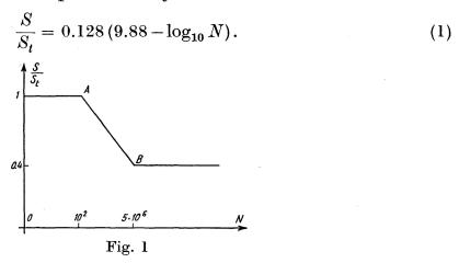
Theories of fatigue damage. There exist many theories concerning the mechanism of fatigue damage. All of them agree that the fatigue damage is a function of the cycle ratio, i.e. the ratio of the number of cycles to which the specimen has been subjected to the total number of cycles representing its fatigue life. The various theories differ in regard to the type of functional relationship that exists between these quantities.
