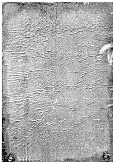
Fig. 18. Poor adhesion of polythene coating to steel.
