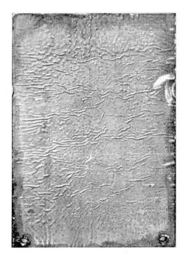
Fig. 18. Poor adhesion of polythene coating to steel.
