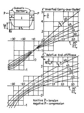
Fig. 3. Hoff's stiffness chart for gusseted member under axial load, rearranged.
