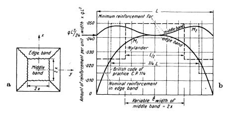
Fig. 14. Collapse of square slabs on stiff beams; required reinforcement according to an upper-bound for the collapse load (equations 11 and 12).
