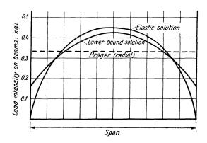
Fig. 15. Comparison of load intensity on beams.
