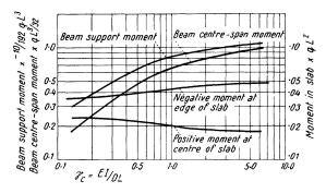
Fig. 10. Beam and slab moments for continuous square panels: all panels carrying a uniform load of intensity q.
