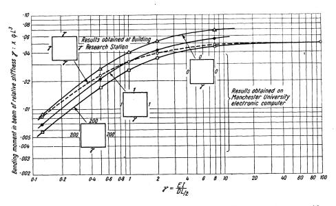
Fig. 8. Bending moments in a beam supporting a square slab carrying a uniform load of intensity q, and the influence of adjacent beams of different stiffness ratios.
