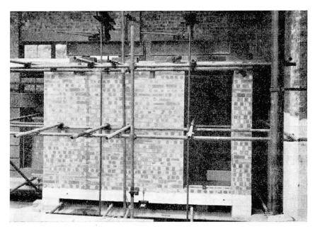
Fig. 3. Vertical loading tests on a cavity brick wall carried by a reinforced concrete beam, with a door opening near the supports.
