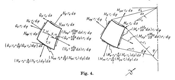
The equilibrium of an element which is cut from the shell by two infinitesimal adjacent meridian and latitude planes gives three equations of summation of projections of forces and three equations of moments with respect to those axis. Hence we obtain the following system of six equations which represent the equilibrium conditions.
