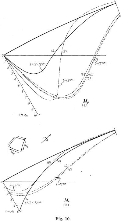
the solution of the second approximation method by M. Hetenyi¹) depending on the average thickness 42 cm. It is seen that this method is sufficiently accurate compared with the exact solution.
