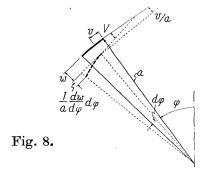
axis of revolution are expressed in the following system by taking account of the transverse shear force and the angle of rotation V of a tangent to a meridian.
