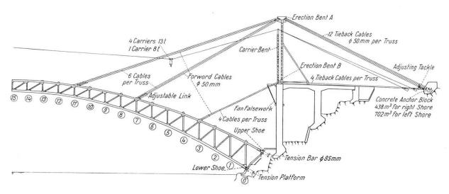
Fig. 4. General view of cantilever tieback system.
