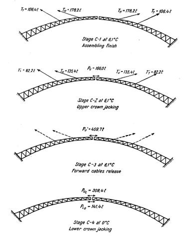
Fig. 9. Process of arch closure.
