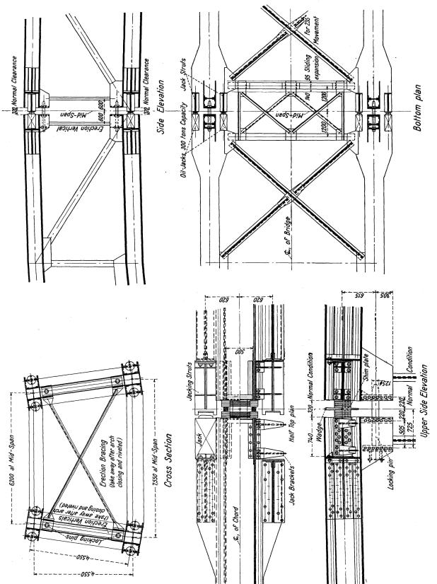
Fig. 8. Details of Crown.
