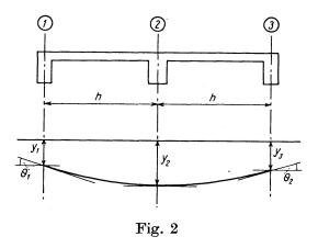
three equal longitudinals, loaded on the centre one, will be worked out. Referring to fig. 2, suppose that the angle of rotation of each outer longitudinal is  $\theta_1$ , then it is easily shown that the shear per unit length of the transverse medium at its connection with girder (1) is
