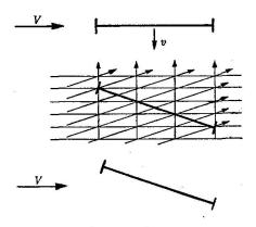
Fig. 11. Tilting of Field of Flow for Vertical Motion of Section. Tilting of Model in Static Wind-Tunnel Tests.
