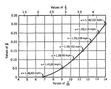
Fig. 22. Instability Graph for Coupled Vertical and Torsional Oscillations. Showing Logarithmic Increment ( $\delta$ ) and coupled Frequency ( $\omega$ ) for Varying Wind Velocities (V/Nb), and Critical Velocities (V/Nb) for Varying Structural Damping ( $\delta$ ). (For Section d/b = 0.02.)
