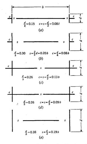
Fig. 29. Aerodynamically Stable Bridge Sections. Combinations of Slots and Fins Provide Complete Aerodynamic Stability.
