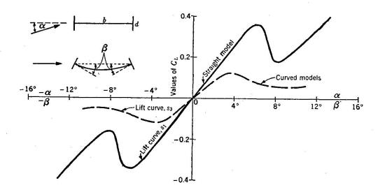
Fig. 13. Static Lift Graphs for Straight and Curved Models of an H-Section (d/b = 0.20).
