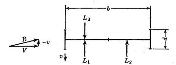
Fig. 10. Aerodynamic Instability of Wide Sections. Lift Resultants for Three Categories of Aerodynamic Stability.
