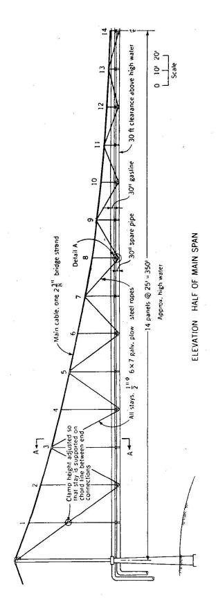
Fig. 6. Pipeline Bridge Stabilized with Diagonal Rope Stays. (Coosa River, Alabama, 1951.)
