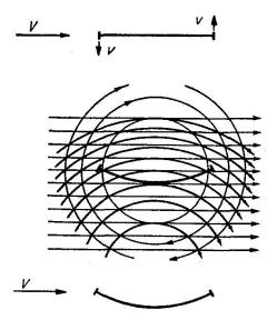
Fig. 12. Curving of Field of Flow for Angular Motion of Section. Derivation of Curved Models for Static Wind-Tunnel Tests.
