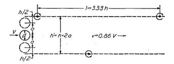
Fig. 4. Vortex Trail in Wake of Oscillating Cylinder.
