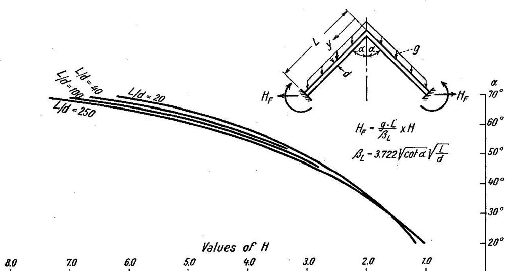
Fig. 8b. Fixed End Reaction — Dead Load
