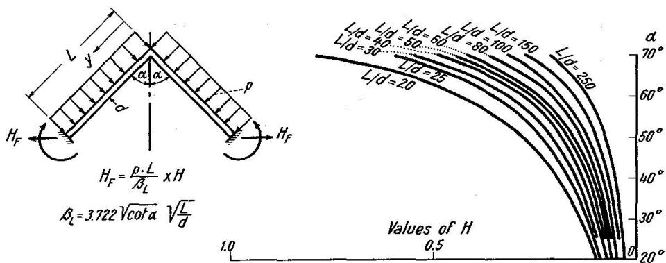
Fig. 10b. Fixed End Reaction — Normal Load
