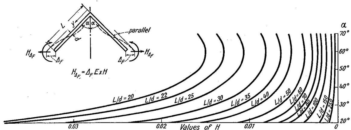
Fig. 7b. Fixed End Reaction due to  $A_F$
