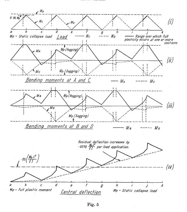
$W_C$ , full plasticity is reached under this load at both A and C (Fig. (II)). Under each application of the load  $W_D$ , full plasticity is reached at both B and D (Fig. (III)). There is no tendency for the range of load over which full plasticity occurs to decrease, and the residual deflections increase progressively (Fig. (IV)).
