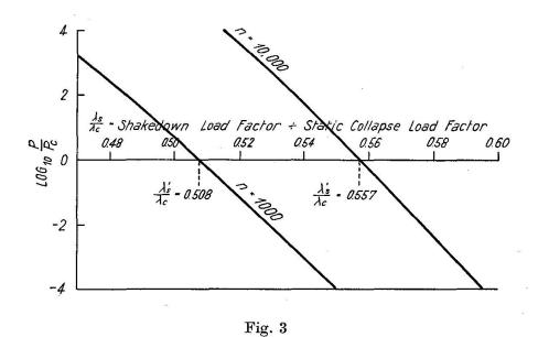
The results are summarised in Fig. 3, in which  $\log_{10}\left(\frac{P}{P_c}\right)$  is plotted vertically against  $\frac{\lambda_s}{\lambda_c}$  horizontally. When  $P=P_c$ ,  $\log_{10}\left(\frac{P}{P_c}\right)=0$ , and hence  $\frac{\lambda_{s'}}{\lambda_c}=0.508$  when n=1000 and 0.557 when n=10,000. If  $\lambda_c=1.75^1$ ), the values of  $\lambda_{s'}$  become 0.890 and 0.975 respectively.
