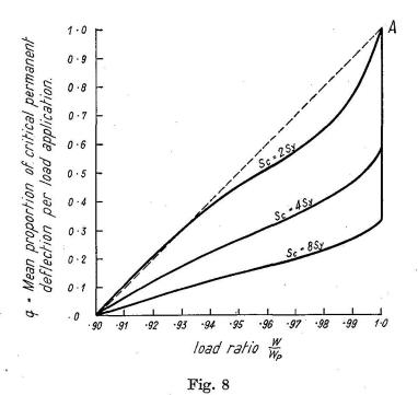
when using the approximate formula by less than 5%. Judging therefore from this particular example, equation (14) appears to give safe results except when the permanent deflection at collapse is assumed to be less than about twice the elastic deflection at yield. Provided deflections in the elastic range are not so
