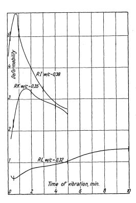
Fig. 4. Effect of variations in the water-cement ratio at a constant cement paste content and a constant grading. The letter symbols refer to the respective mixes and the vertical dashes mark the times of vibration in the tests described in Section B
