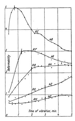
Fig. 5. Effect of variations in the percentage of cement paste at a constant water-cement ratio and a constant grading. The figures above the curves express the cement paste content in per cent by solid volume. The letter symbols refer to the respective mixes and the vertical dashes mark the times of vibration in the tests described in Section B
