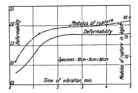
Fig. 8. Example of correlated deformability and strength curves
