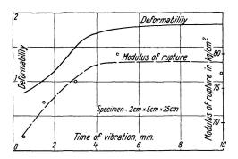
Fig. 9. Example of correlated deformability and strength curves
