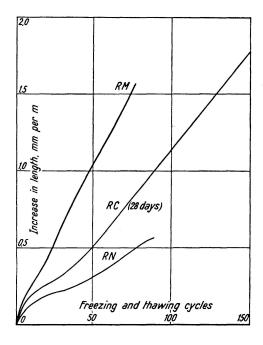
Fig. 16. Increase in length in freezing and thawing tests. Test series No. 4. The mix RC had similar proportions to the mix RO, but the test specimens were water-cured for 28 days. (For the mixes RM and RN, the curing time was only 7 days)
