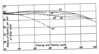
Fig. 15. Change in modulus of elasticity in freezing and thawing tests. Test series No. 2
