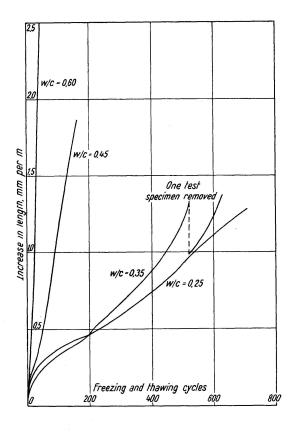
Fig. 10. Increase in length in freezing and thawing tests. Varying water-cement ratio, constant grading, and constant deformability
