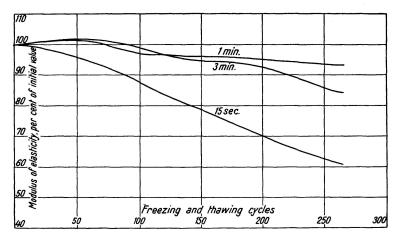
Fig. 22. Effect of variations in time of vibration on the change in modulus of elasticity in freezing and thawing tests. Mix RI
