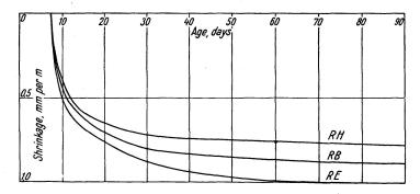
Fig. 23. Shrinkage of mixes in the test series No. 2
