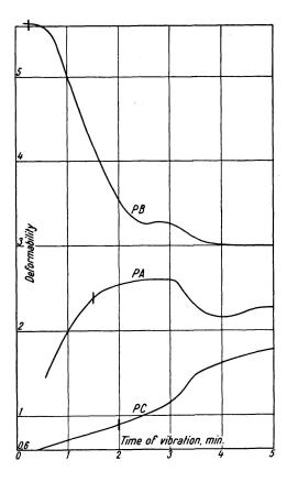
Fig. 24. Deformability curves of mixes for creep tests. The vertical dashes mark the times of vibration in the preparation of test specimens
