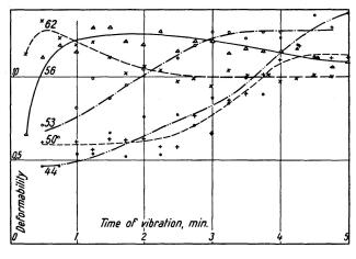
Fig. 6. Effect of variations in grading at a constant water-cement ratio and a constant cement content. The figures above the curves express the amount of coarse aggregate in per cent of the total aggregate
