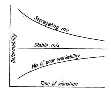
Fig. 2. Characteristic types of deformability curves
