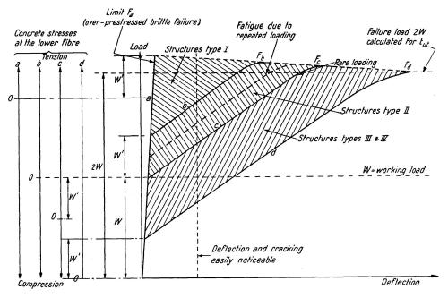
Fig. 1. Different types of structures, load deflection diagrams
