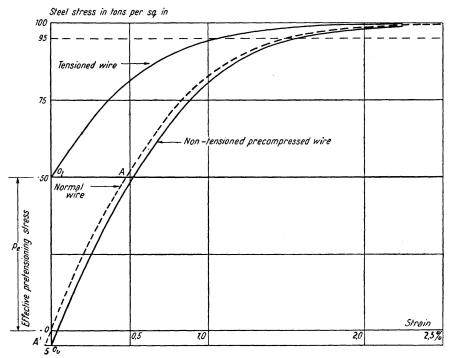
Fig. 2. Stress strain diagrams of wire 0.2 in. (5 mm) dia.
