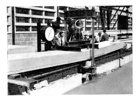
Fig. 4. Static test on partially prestressed composite slab, 1951
