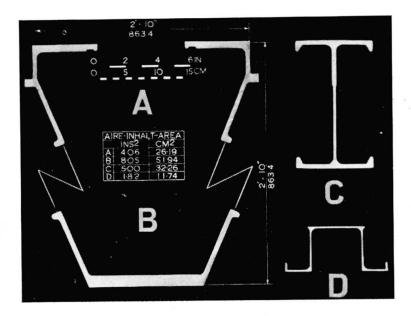
Fig. 6. Extrusions for Ribs, Rafters and Purlins
