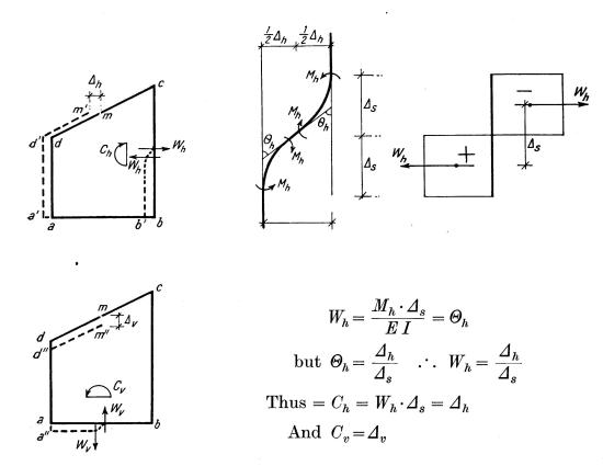
Fig. 12. The Elastic Couples  $C_h$  and  $C_v$
