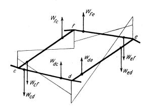
Fig. 8a. Equilibrium of the Elastic Weights in a Closed Panel
