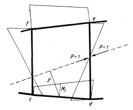
Fig. 8b. The Moment Diagram of the "Free Main System"
