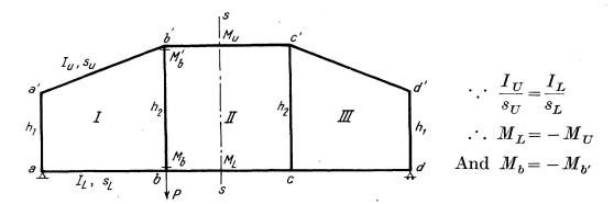
Fig. 13a. Vierendeel Girder of Equal Chord Stiffness
