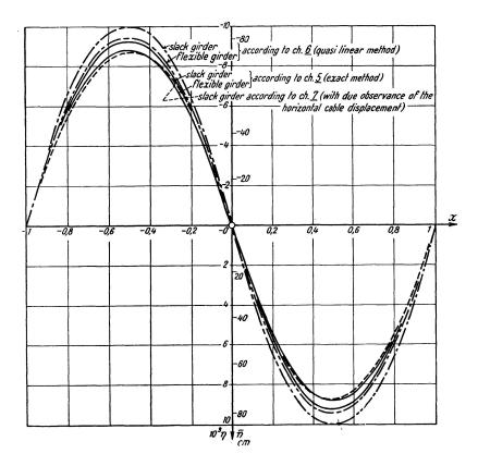
Fig. 3. The girder deflection with an inextensible cable, a constant live load being placed on one of the two halves of the girder
