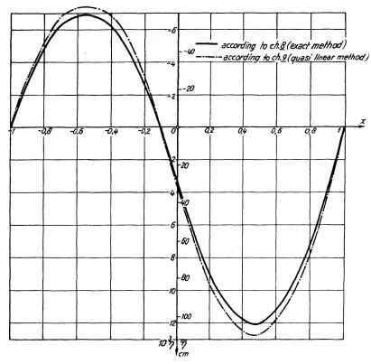
Fig. 6. The girder deflection with an extensible cable and a constant live load placed on one of the two halves of the girder
