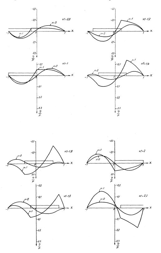
Fig. 15b. The girder deflection as a function of x and vt with a moving load, uniformly distributed
