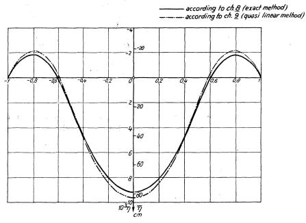
Fig. 7. The girder deflection with an extensible cable and a constant symmetrical live load extending over half the girder
