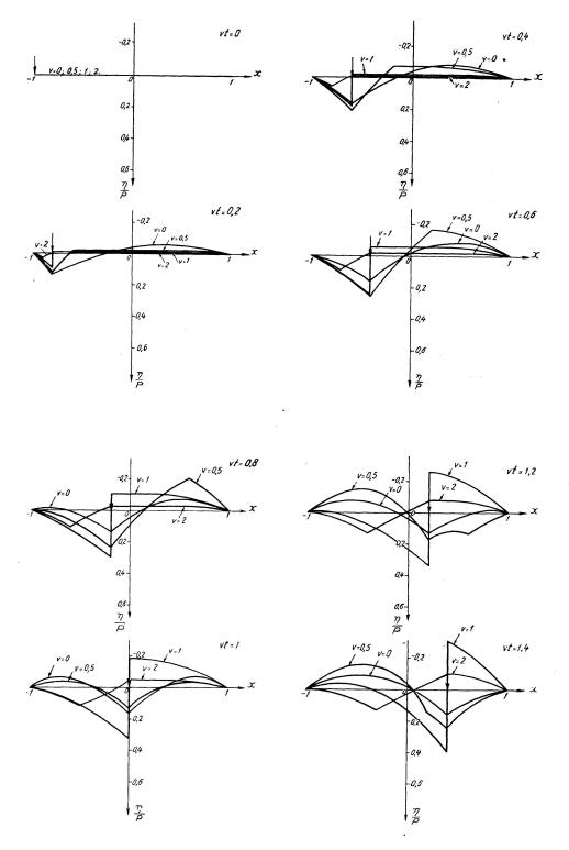
Fig. 13a. The girder deflection as a function of x and vt with a moving concentrated load
