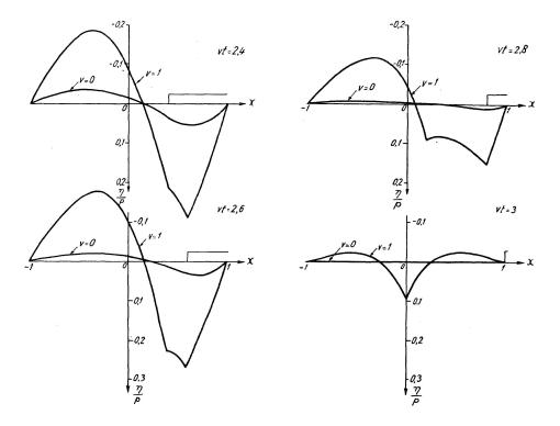
Fig. 15c. The girder deflection as a function of x and vt with a moving uniformly distributed load
