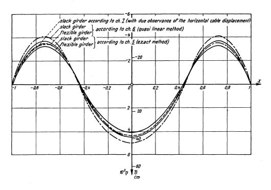
Fig. 4. The girder deflection with an inextensible cable and a constant symmetrical live load extending over half the girder
