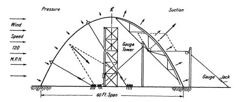
Fig. 5. Diagram showing arrangement of test straining devices
