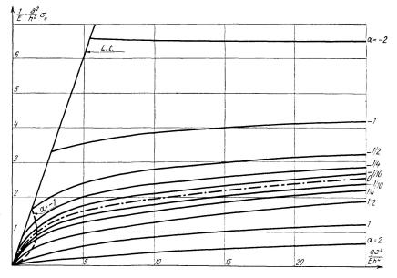
Fig. 14. Bending stress at the centre of the plate as a function of the load for various values of the initial deflection in Example No. 4b. For small values of  $\frac{q a^4}{E h^4}$  and negative values of  $\alpha$ , a curve is given only for  $\alpha = -1$ . L.t. = the bending stress calculated in accordance with the linear theory of plates
