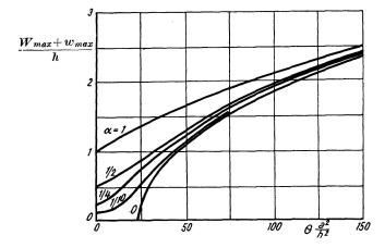
Fig. 5. Deflection at the centre of the plate in Example No. 2 as a function of  $\theta \frac{a^2}{h^2}$  for various values of the initial deflection (for the angle  $\theta$ , see Fig. 4). The curve for  $\alpha = 0$ , initially plane plate, has been calculated by Bergman. The initial deflections are included.
