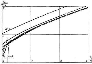
Fig. 18. Maximum bending stress occurring in the plate as a function of the external load at various values of the initial deflection in Example No. 5
