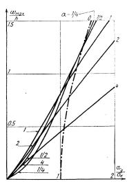
Fig. 16. Deflection at the centre of the plate as a function of the radial compressive stress applied along the external circumference in Example No. 5 for various values of the initial deflection. The curve for the initially plane plate has been calculated by FRIEDRICHS and STOKER
