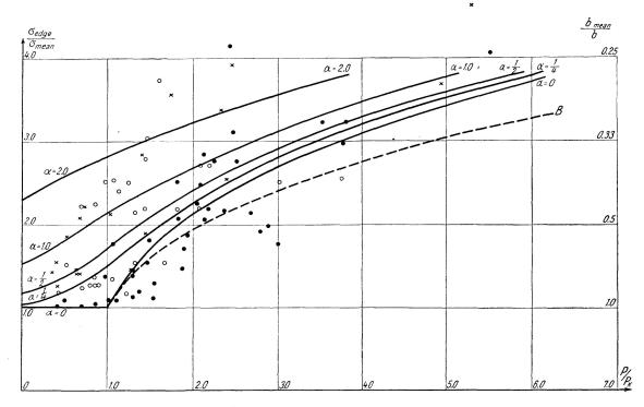
Fig. 10. Test values of  $\frac{\sigma_{edge}}{\sigma_{mean}} \left( \frac{b_{mean}}{b} \right)$ plotted in relation to the curves for various values of the initial deflection.
