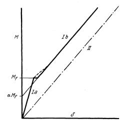
Fig. 6. Theoretical shape of deflection curve. The short-dash line curves indicate the approximate actual shape of the upper limit curve
