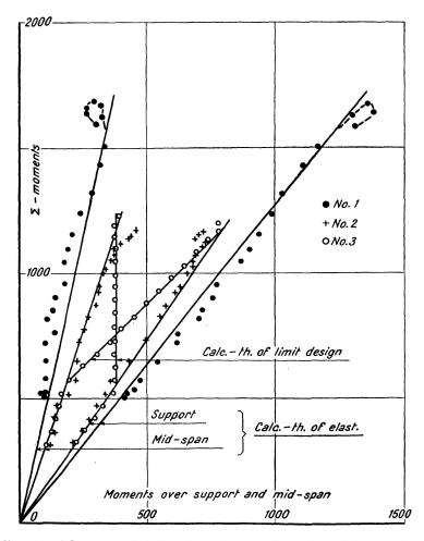
Fig. 14. Moment distribution observed at the ultimate load
