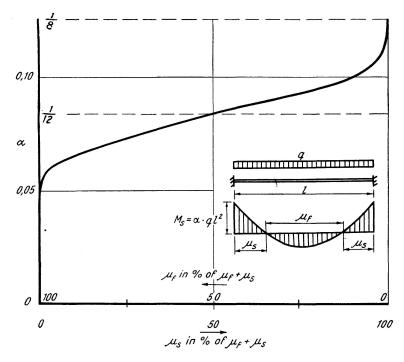
Fig. 9. Calculated variation in the moment at the support with the distribution of reinforcement at the supports and between the supports ( $\mu = \text{ratio of reinforcement}$ )
