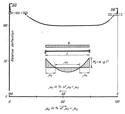
Fig. 10. Calculated variation in deflection with the distribution of reinforcement at the supports and between the supports ( $\mu = \text{ratio of reinforcement}$ )
