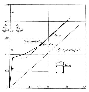
Fig. 3. Comparison of strains observed in tension tests on reinforced concrete prisms<sup>2</sup>) and calculated from Eq. (6)
