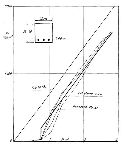
Fig. 5. Comparison of stresses in reinforcement observed in tests<sup>4</sup>) and calculated from Eq. (17a)
