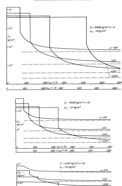
Fig. 8. Calculated limit curves for the idealised modulus of elasticity. The full-line curves represent the upper limit, whereas the dash-and-dot line horizontal asymptotes correspond to the lower limit ( $\sigma_s$  in kg/cm<sup>2</sup>)
