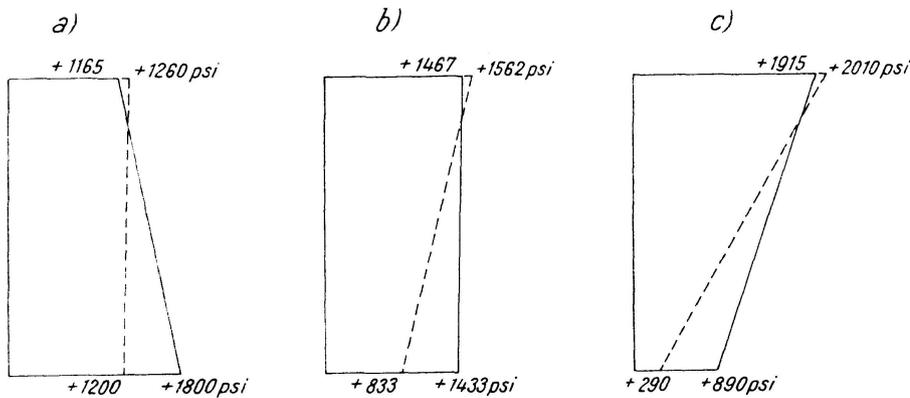
Fig. 7. Typical Stress Diagrams for Midspan Section
