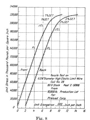
Stress Strain Curve of Roebling 0,276" Wire
