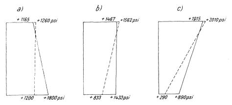
Fig. 7. Typical Stress Diagrams for Midspan Section
