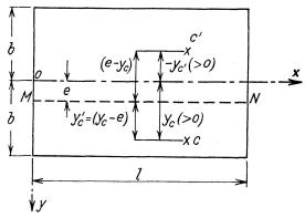
$$w(y) = c_m e^{-m\omega \sqrt{\frac{1+\alpha}{2}}|y-e|} \sin \frac{m\pi x}{l} \left\{ \cos \left[ m\omega \sqrt{\frac{1-\alpha}{2}}|y-e| \right] + \sqrt{\frac{1+\alpha}{1-\alpha}} \sin \left[ m\omega \sqrt{\frac{1-\alpha}{2}}|y-e| \right] \right\} \quad (y \ge e)$$
