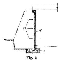
The backing of stabilised soil may now be constructed, the soil being hand rammed carefully round the anchor ties and consolidated by rolling elsewhere. The supporting struts should be left in place for several days after the completion of the backing, after which they may be removed and the superstructure work may proceed.
